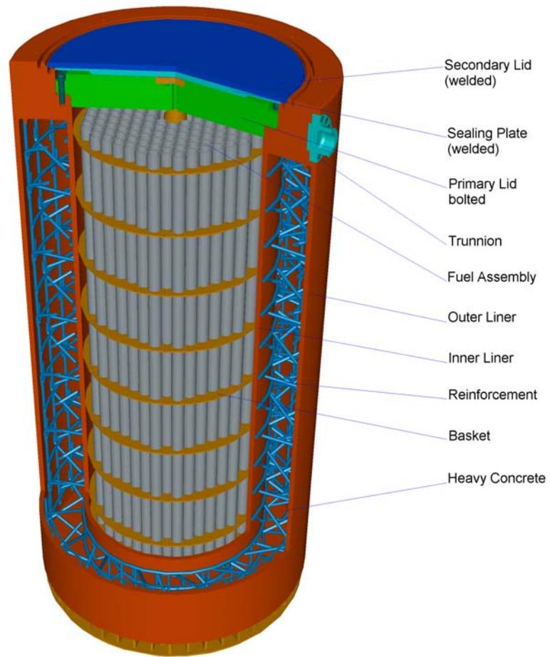
**Fig. 3. Multipurpose Constor<sup>®</sup> Storage, Transport, and Disposal Cask.**
