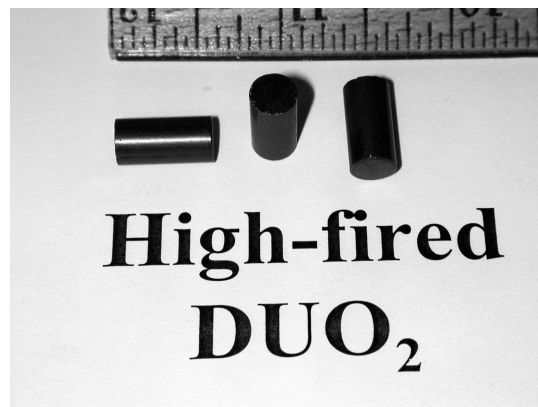
Fig. 2. High-fired DUO 2 pellet.
