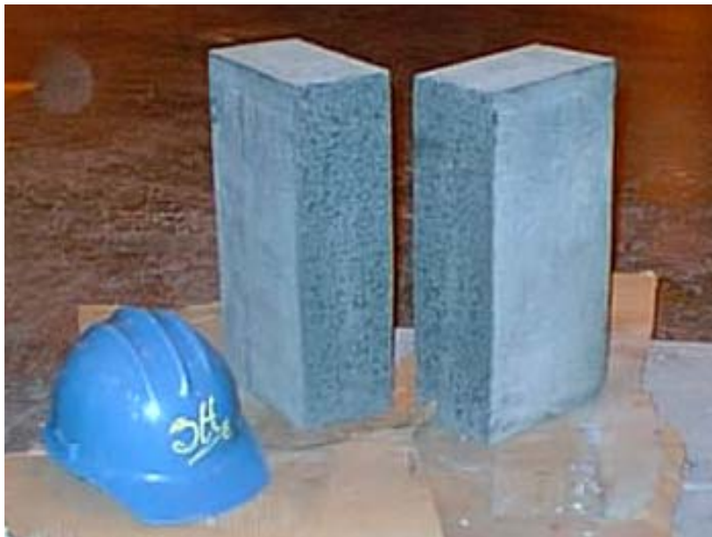
Test block sectioned after curing
